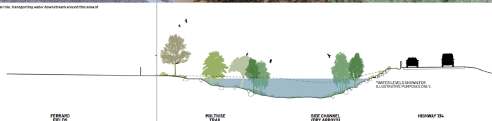
Figure 378. In this design example, the Ferraro Side Channel accommodates large, infrequent storm events by filling up with flood waters and downstream through a side channel that bypasses the bend in the river near Shandera.
